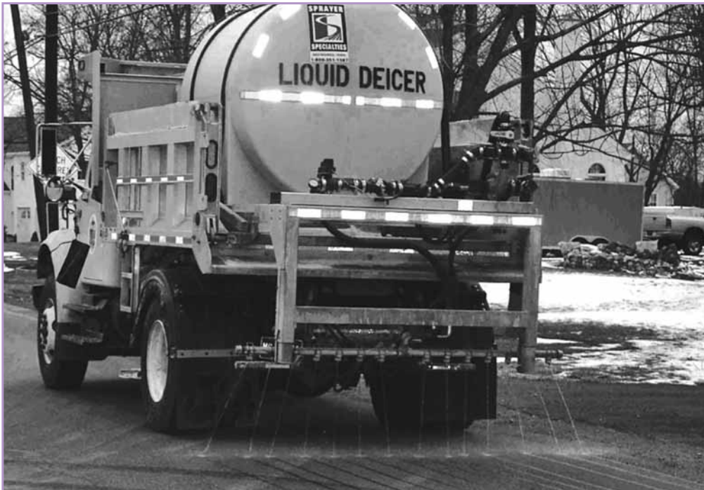
Plow truck applies application of brine solution on Church Road
