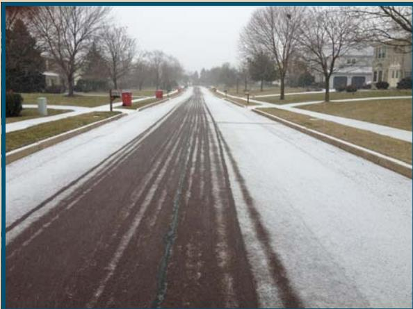
Bringing in advance of storms continues to be an efficient method to prevent snow and ice from bonding to the road surface.
