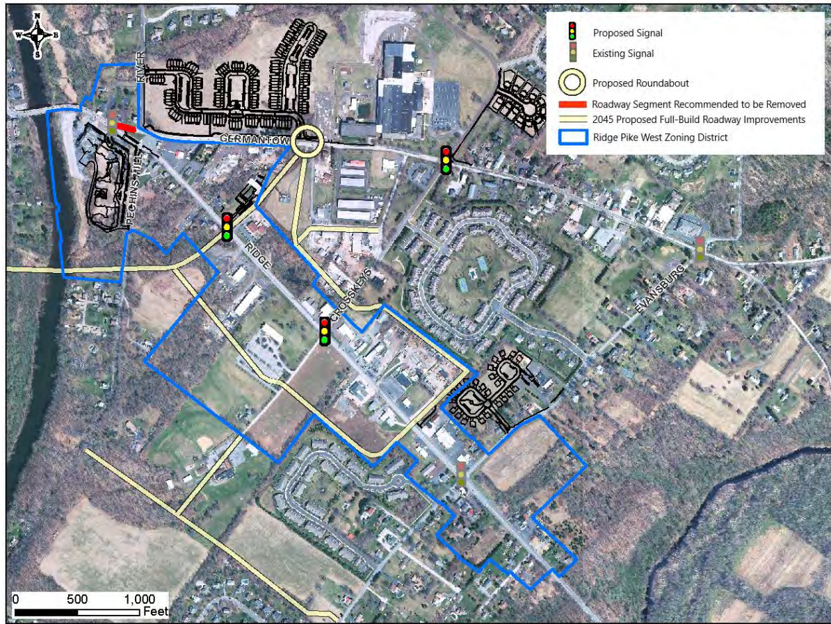
Figure 18 Recommended Long-Term Roadway Improvements
